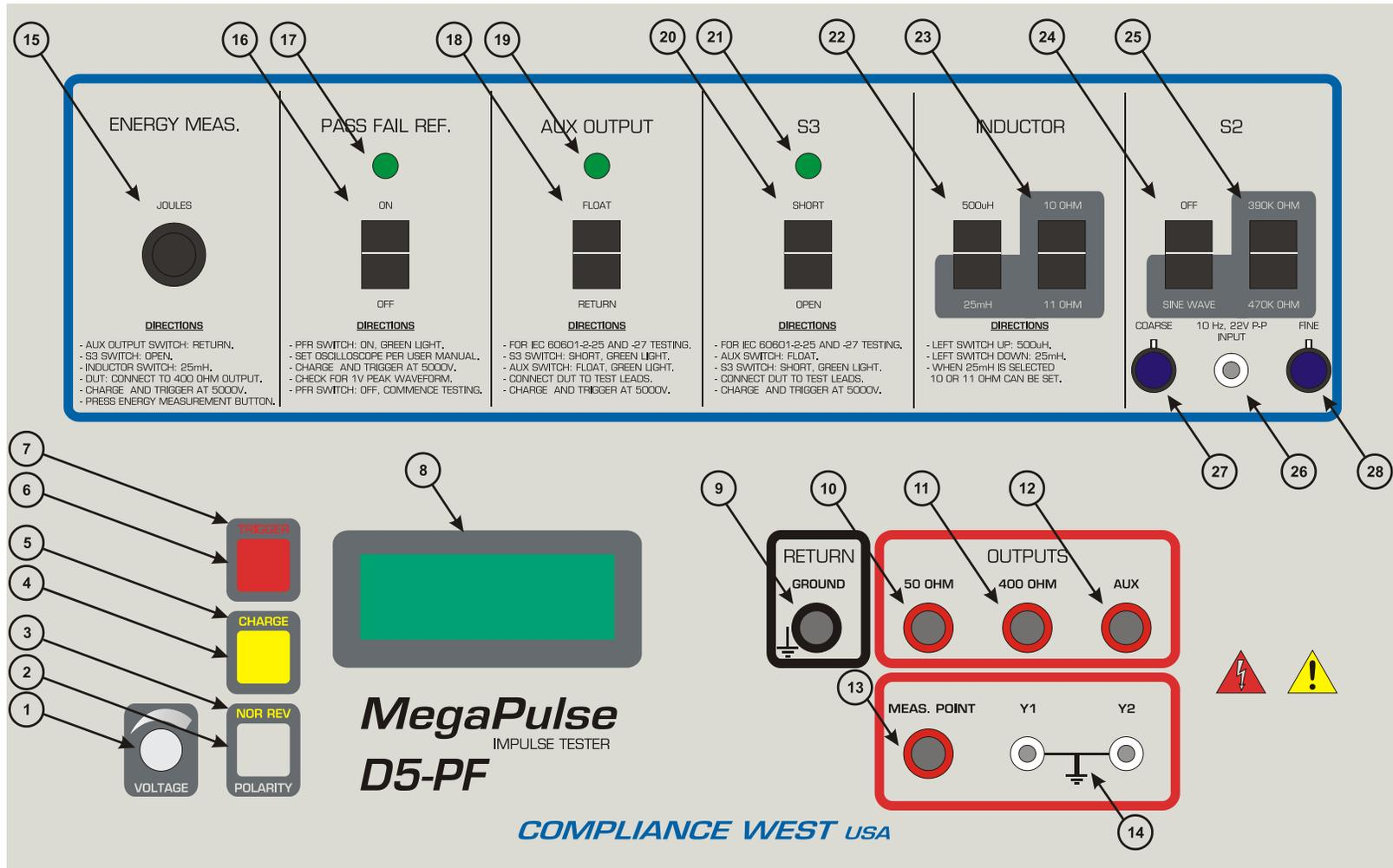
Figure 1 Controls, Indicators, Connectors – MegaPulse D5-PF Front Panel
