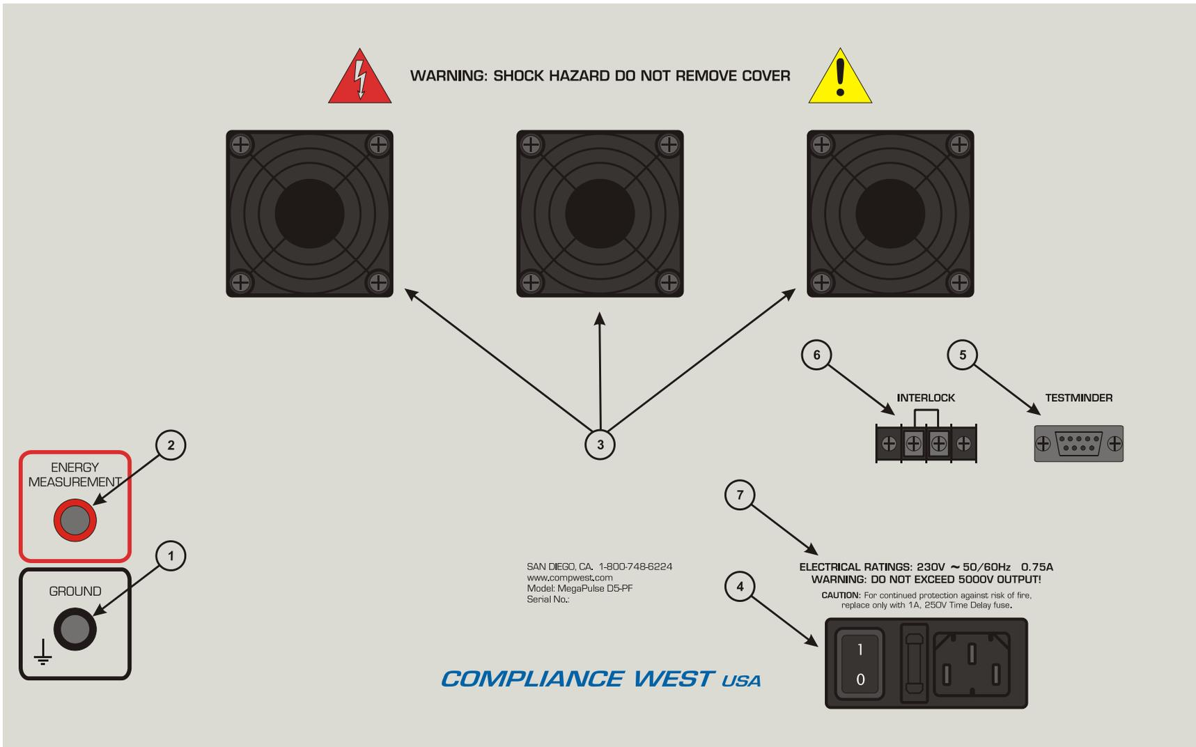
**Figure 2. Controls, Indicators, Connectors – MegaPulse D5-PF Rear Panel**
